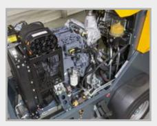
The powerful three-cylinder Deutz engine boasts 55.4 kW thanks to the charge-air cooler and meets all requirements of the "Stage V" emissions standard, applicable in the EU and Switzerland.
