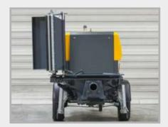
The larger folding hopper with rubber collar (360 l), protective grille and splash guard (option) offers perfect protection against concrete spatter.
