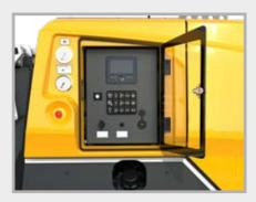
The central operating panel with intuitive keypad employs the "follow the blue light" principle, is easy and safe to operate and is well protected by a robust acrylic-glass door.
