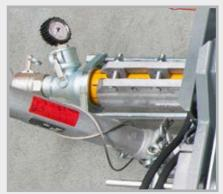
The powerful 2L6 worm pump with M 50 pressure connection is included as part of standard equipment. It can process sitemade mixes with up to 6 mm grain size, depending on the desired delivery rate and the properties of the material.
