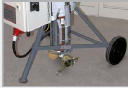
Discharge connection with pressure gauge for connecting mortar hoses
