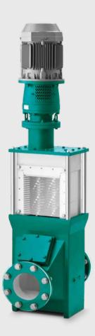
The NETZSCH twin shaft macerator provides a free flow through, protecting the pumps and other plant equipment. Depending on the application one of five different models and sizes can be installed. Through the different, very low number of revolutions of the shafts the NETZSCH twin shaft macerator offers the option of self cleaning. Low power drives can be used even on high throughput applications.
